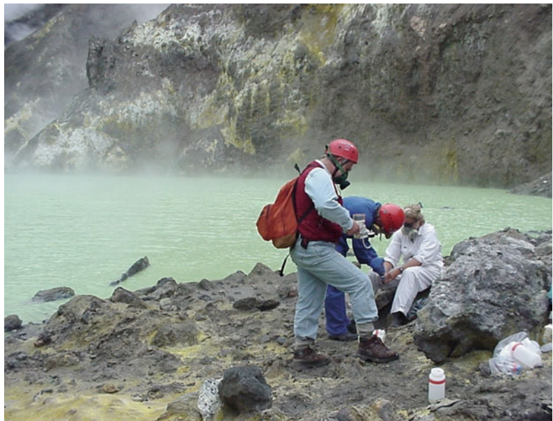
Fig. 2 Sampling at White Island, New Zealand. Acidic gases require use of respirators. The water’s green coloration is due to elemental sulfur. (Photo SPD)
